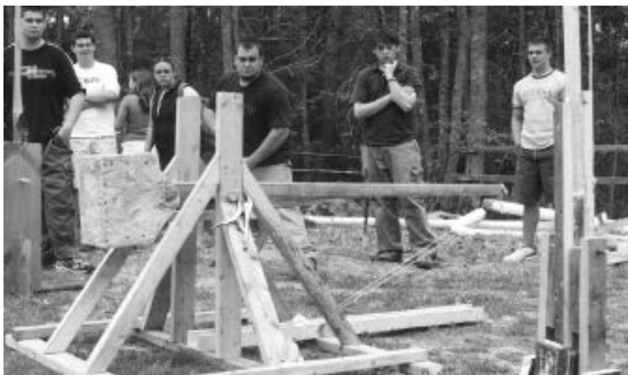
Physics student Brandon Warstler '03 launches a golf ball from his trebuchet to measure distance and accuracy and assess his design
